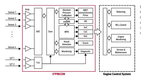
E<sup>2</sup>PRECON-M computes IMEP, peak pressure, heat release, combustion timings and knock levels for each cylinder and every engine working cycle. This data is transmitted synchronously to the engine control system where it is used for various purposes.
